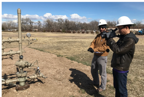
Figure 2-1. FLIR GFx320 OGI camera (left) [31], and similar camera in use at the Methane Emissions Technology Evaluation Center (right) [32].
